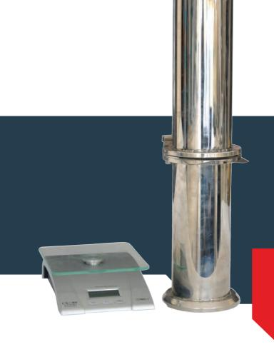
Measures hectoliter of grain which is the weight of a 1 liter of kernel.
