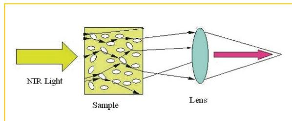
Within this region of the electromagnetic spectrum, N-H (protein), C-H (fats and oils) and O-H (water) and C-O-H (carbohydrates) absorb NIR light at specific frequencies. The NIT spectrum contains information about the concentration of these components. Calibration models, stored in the CropScan's computer, converts this information to % Protein, % Moisture, % Oil and % Starch and displays the results on the screen.
