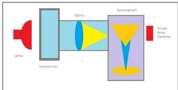
The separated light is then directed onto a silicon photo diode array detector. This array detector measures the intensity of the light at each frequency to produce what is called the NIT spectrum of the sample.
